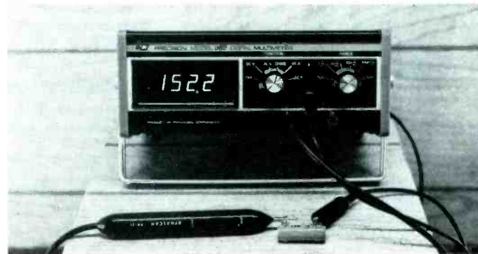
Read-out of 3-1/2 digits plus stable and accurate circuitry shows this resistor to be 152.2 ohms, not 150 or 160 ohms.
